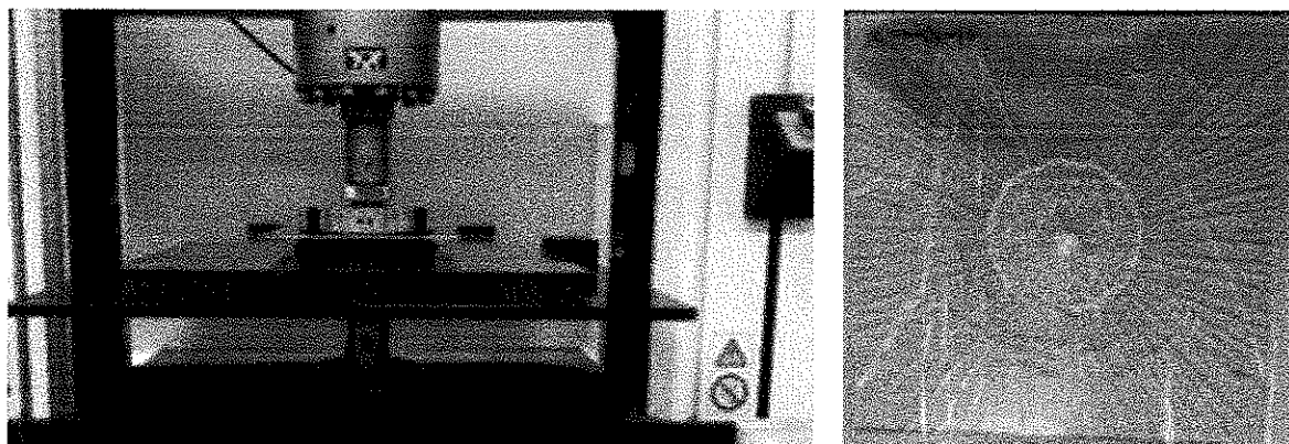
Fig. 2: Coaxial double rings (CDR) test method and corresponding crack pattern.
