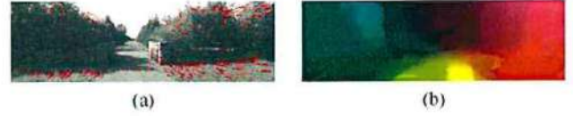
Fig. 2. Optical flow fields a) feature based (sparse) b) intensity based (dense).
